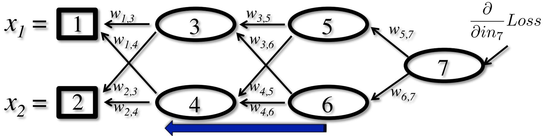
$$\frac{\partial}{\partial in_j} Loss = g(in_j)(1 - g(in_j)) \sum_k w_{j,k} \frac{\partial}{\partial in_k} Loss$$
